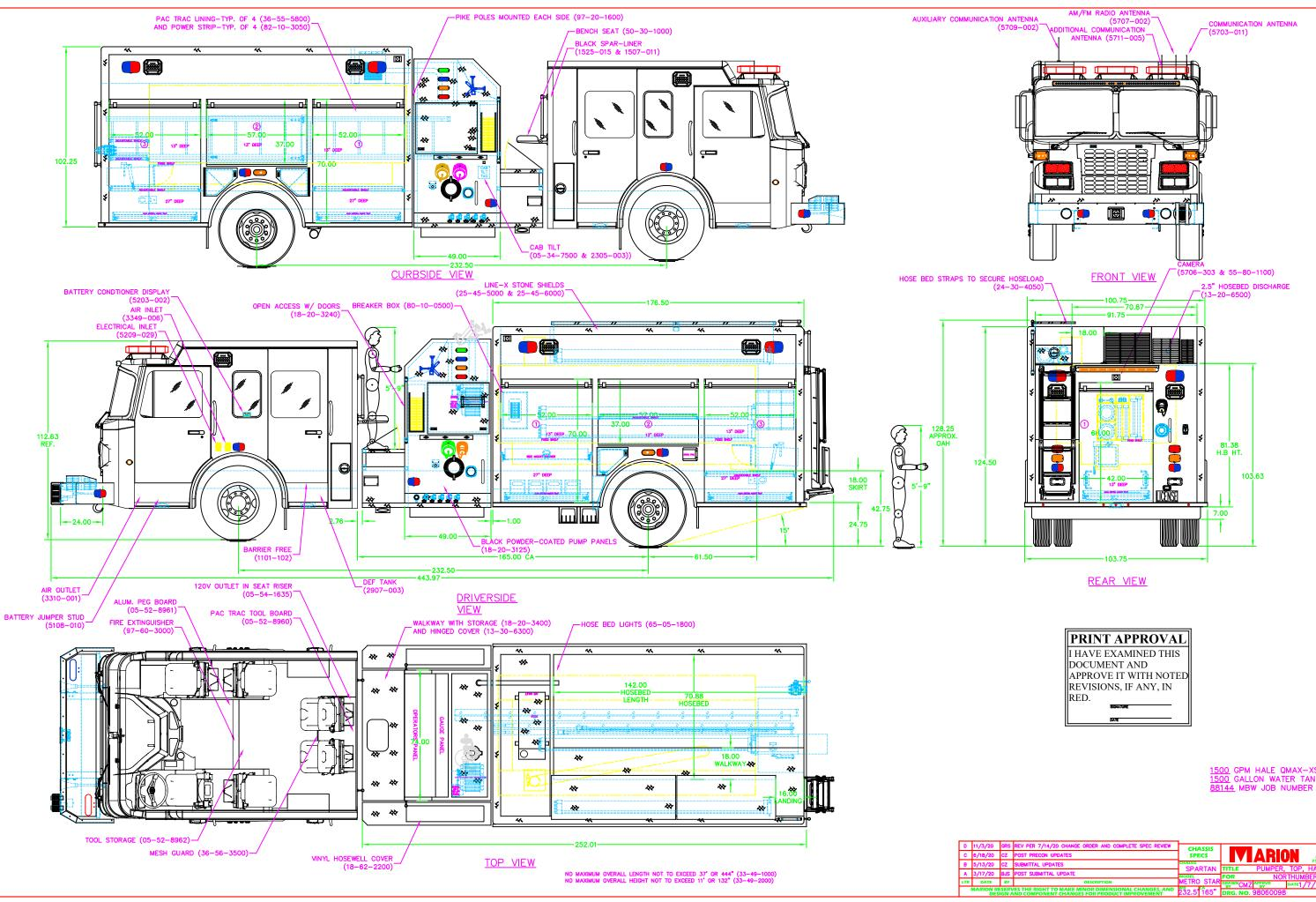
1500 GPM HALE QMAX-XS PUMP 1500 GALLON WATER TANK 88144 MBW JOB NUMBER
